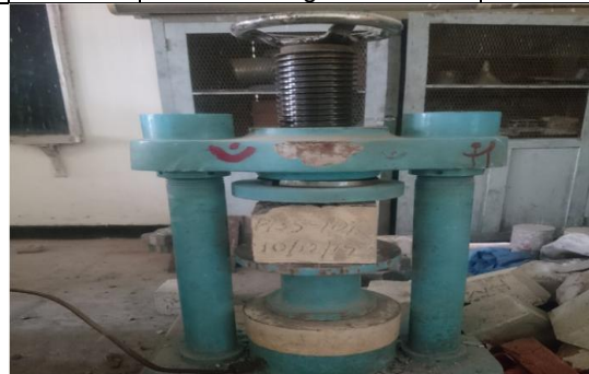
Fig4: During Compression Test of the Cubes
